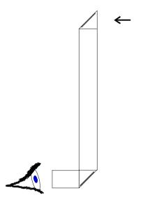
Copy this diagram onto a large bristol board (it'll be better if it's black on the inside), stick two mirrors in the positions you see in the image below, trim the bristol board and set up your periscope.
